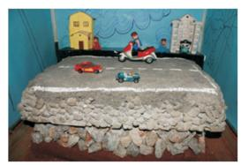
Pervious concrete is traditionally used in parking areas, areas with light traffic, residential streets, pedestrian walkways, and greenhouses. To prevent reduction in permeability, pervious concrete needs to be cleaned regularly. Cleaning can be accomplished through wetting the surface of the concrete and vacuum sweeping.
